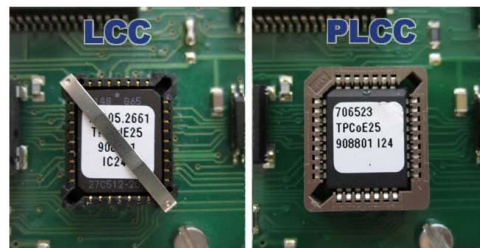
Figure 2: EPROMS on the Control Boards
